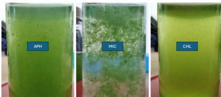
Clarification in Aphanizomenon (APH), Microcystis (MIC) or Chlorella (CHL) suspensions 5 minutes after addition of clay polymer nanocomposites at doses equivalent to neutralize only 25% of the relevant charges.
